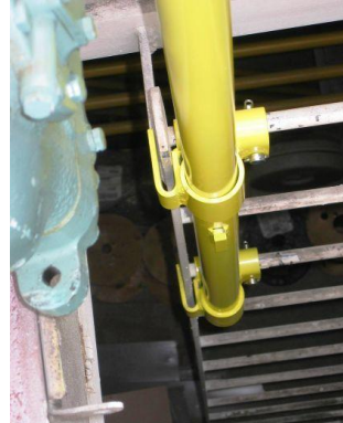
Port-A-Post On Hatch Ladder
